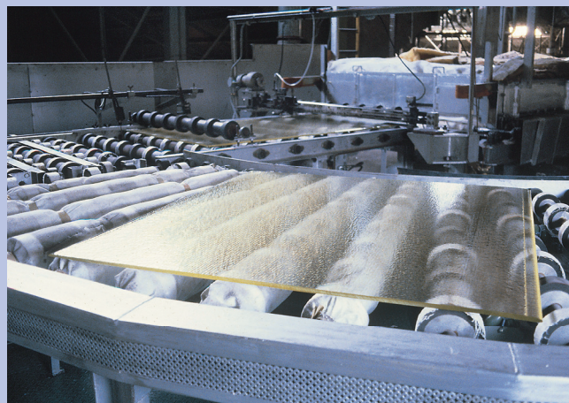
The large-size LX-57B (max. 1,200 x 2,600 mm) produced by continuous production process.
